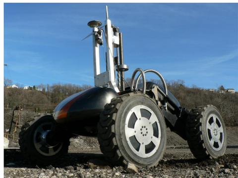
Figure 2: Carnegie Mellon University's Scarab robot. Mast mounted scanning lidar sensors map the terrain for obstacle detection. (Photo: CMU)
