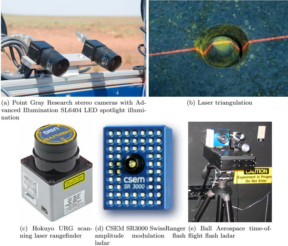
Figure 6: Terrain hazard detection sensors
